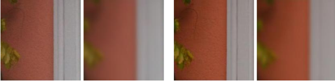
Figure 5: Fragments from the original and blurred images taken by the phone (two left-most) and DSLR (two right-most) camera. Blurring removes high-frequencies and makes color comparison easier.
