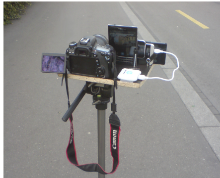
Figure 2: The rig with the four DPED cameras from Table 1.
