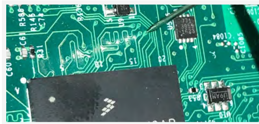
Figure 60. Probing vias with a needle
